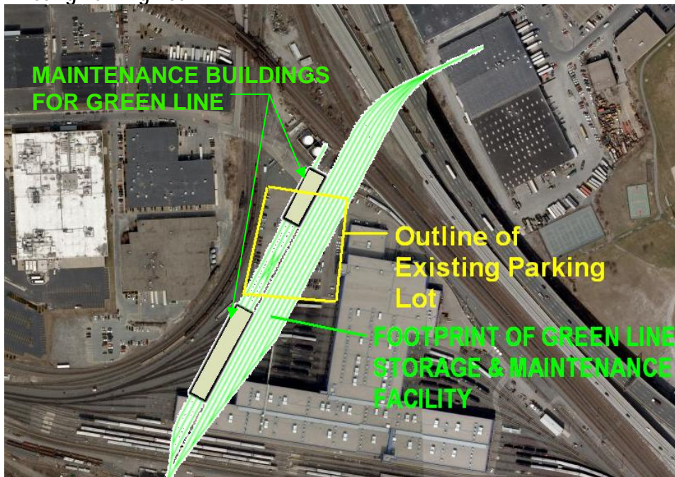
Figure 3: Comparison of Footprint of Green Line Yard with Footprint of Existing Parking Lot
